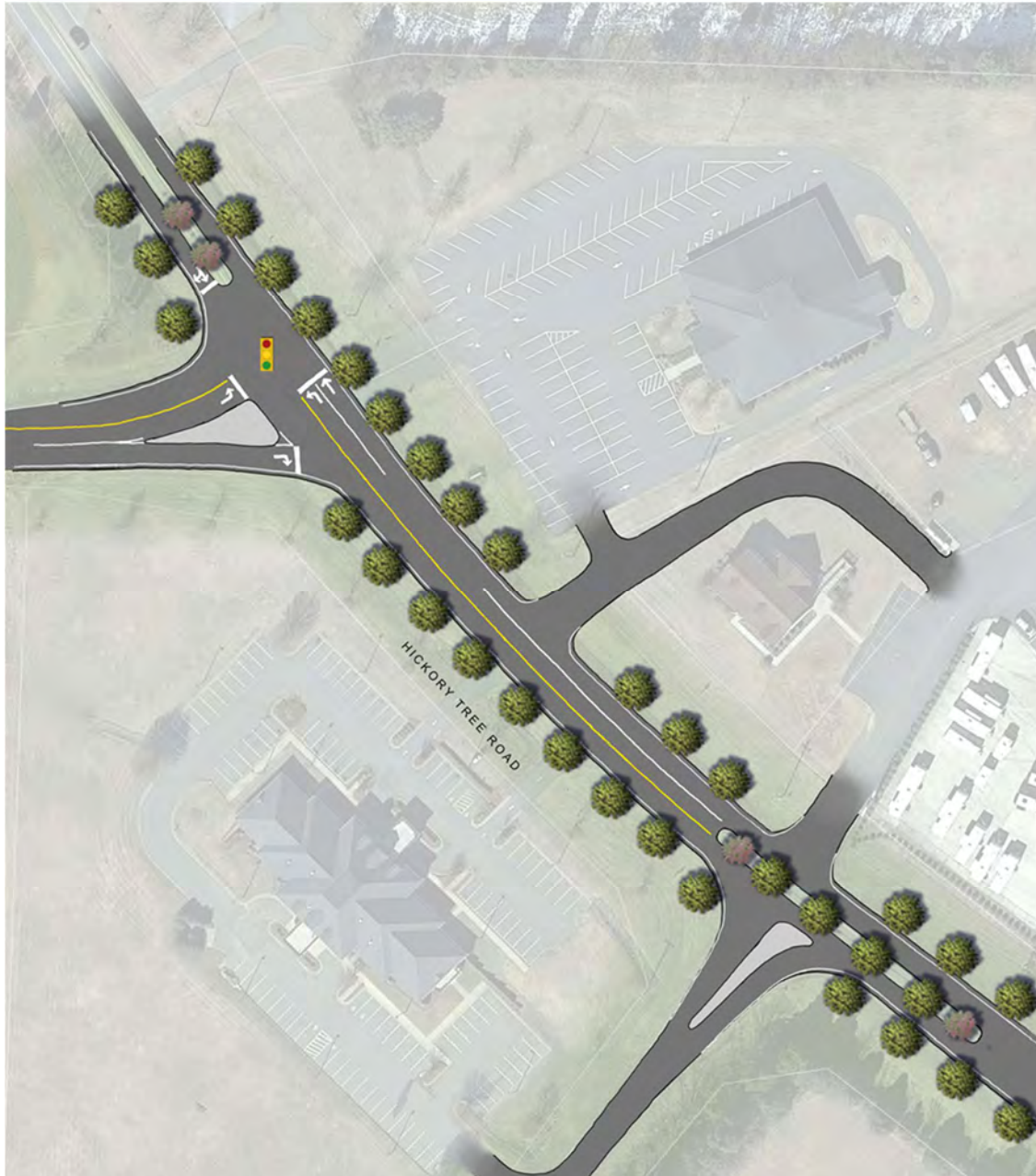
Concept Design of the Signalized intersection Concept for Hartman and David Smith Road.
